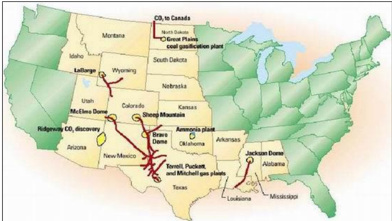
Figure 2: Carbon Dioxide Pipelines in the U.S. 185
